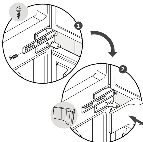
Once the product is attached to the cabinet through the bracket, place the hinge cover, push it until you hear a 'clap'.
