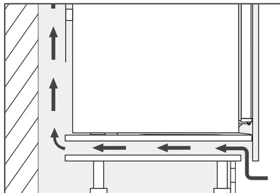
In case it is not possible to make an opening in the baseboard, find an alternative solution to ensure air circulation.
