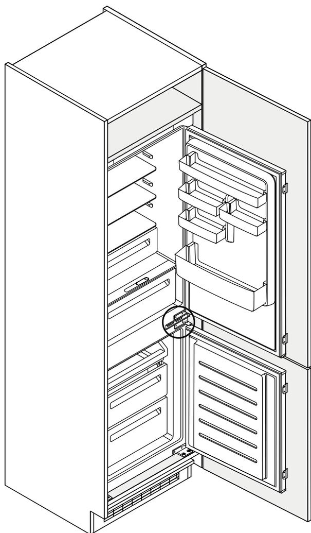
Using the supplied bracket, attach the product to the sidewall.
