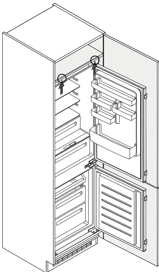
Using the provided screws, attach the upper faceplate to the cabinet shelf and close with the covers.
